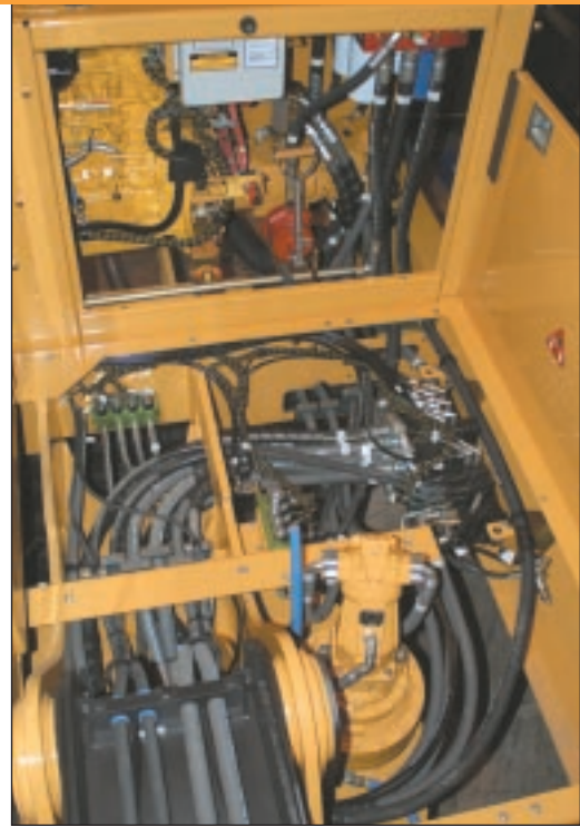
All Tigercat loaders offer walk-up platform access to the cab, engine enclosure, valves and planetary gearbox.
