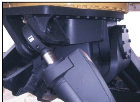
Super-duty leveling system with large pins and cylinders and thick steel plate
