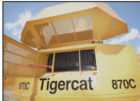
Rear air intake away from saw debris
