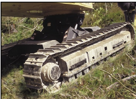
Long track frames and wide stance carbody for excellent stability on slopes
