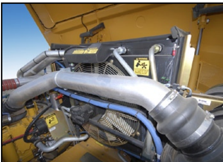
High capacity variable speed cooling
