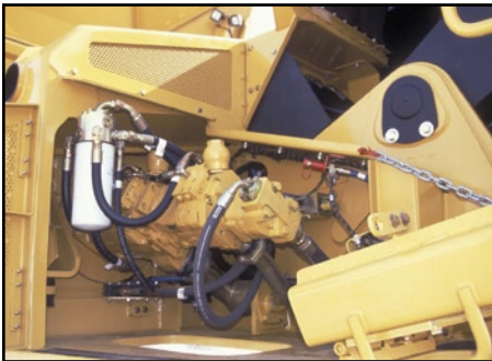
Separate, easily accessed pumpstack
