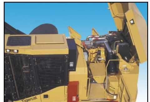
Easy access to the components through hydraulically retracting hood enclosure
