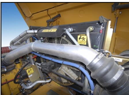
High capacity variable speed cooling
