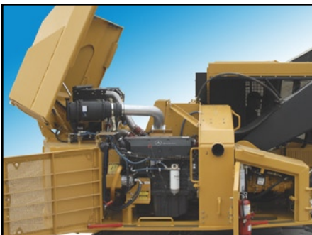
Easy access to engine service points
