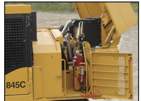
Clamshell style retracting roof enclosure
