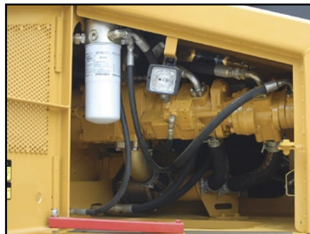
The pumpstack is housed in a separate compartment
