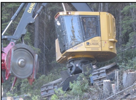
LX model with closed loop track drives for high performance on slopes
