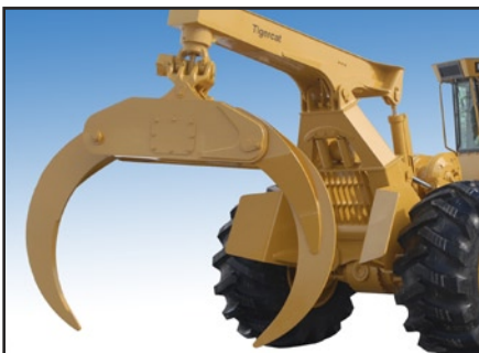
High capacity dual cylinder Tigercat grapples with large tip-to-tip opening
