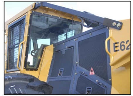
Clear sight line to the sides of the engine compartment
