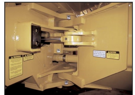
Strong centre section with large pins and tapered roller bearings
