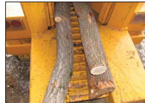
Wide track-type infeed conveyor
